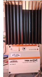
Solar Charge Controller
