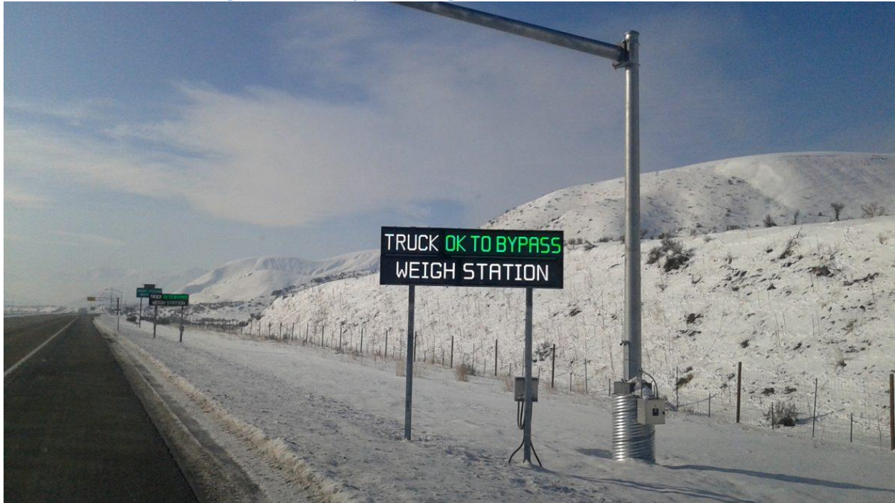
Figure 2-12: Example of a Weigh Station Pre-Selection Board
